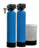
Automatic system for the treatment of steam boiler make-up water, designed to prevent scale deposits and corrosioncaused by dissolved gases. The treatment includes a softening process by means of ion-exchange resins and the chemical elimination of oxygen by dosing a conditioning product.
